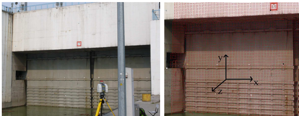
Figure 2 - Location of the Leica HDS3000 system during experiment on the left and position of measured points and selection of coordinate system on the right
